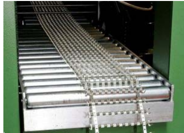
Telecom products are now made in one step rather than in separate blanking and forming operations
